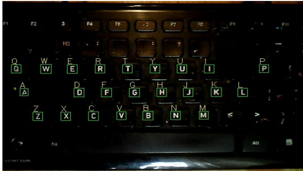
Figure 9. Result of letter identification by the keyboard detection algorithm
