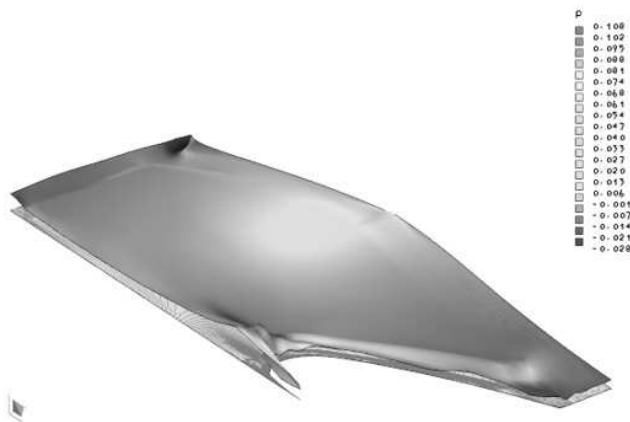
Figure 4. The liner cumulative jet formation and stress tensor values disposal
