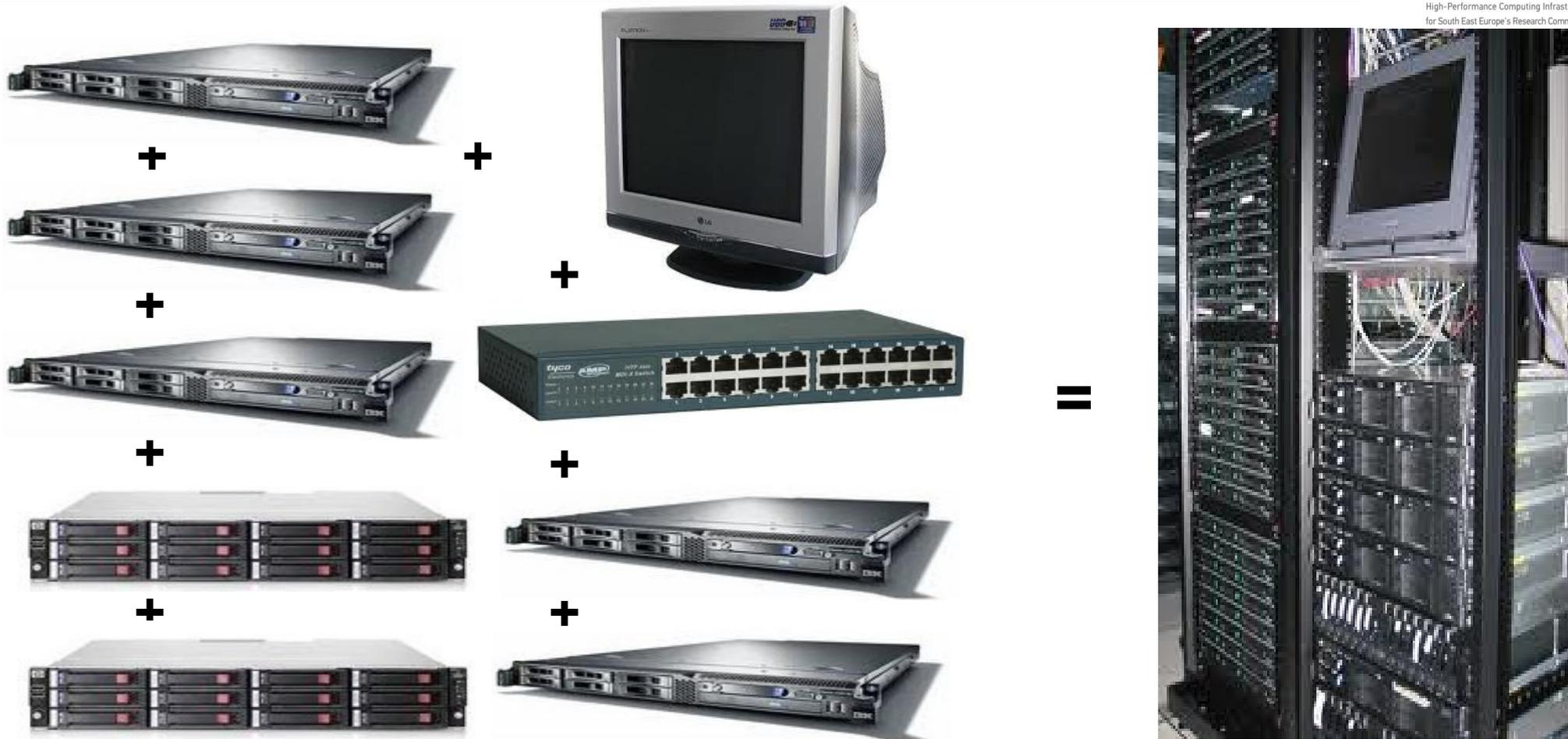
A **cluster** is a group of computers connected by high-speed communication channels (1-2 Gbit/s) and representing, from a user's point of view, a single hardware resource.
