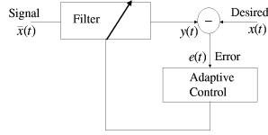
Figure 9. The Adaptive Filter Model
