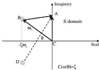
Figure 7. Key Components in The Poles and Zeros Plot of a Second Order Filter
