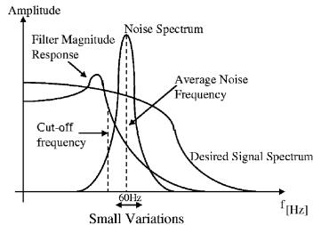
Figure 8. Adaptive filtering under a spectral overlap between a signal and a strong interference
