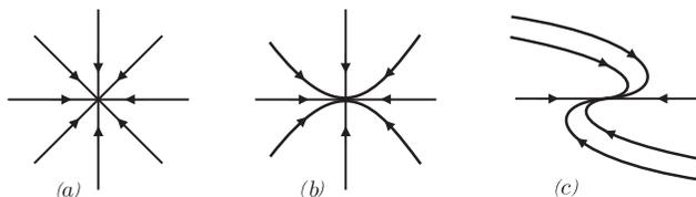
Figure 1. Different types of nodes
